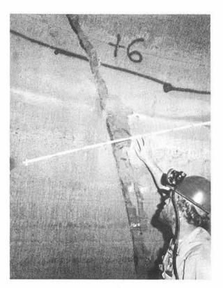
BILL VOLLENDORF (1133) examines a crack produced by hydraulic fracture experiment in the volcanic tuff of G-tunnel at NTS. Bill directs field operations for Sandia's Geophysical Laboratory at NTS.
